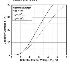
Figure 5. Saturation Voltage vs. Case
