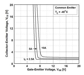
Figure 7. Saturation Voltage vs. V<sub>GE</sub>
