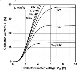
Figure 3. Typical Saturation Voltage Characteristics
