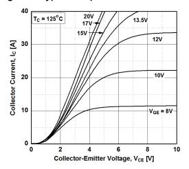
Figure 4. Transfer Characteristics
